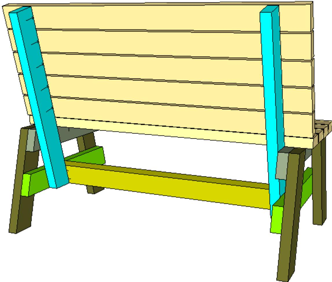
**\*\*TIP\*\*** - Draw a line down the front of all of your back slat where the slats will be screwed into the (blue, vertical) 2x4. This will eliminate guesswork.
